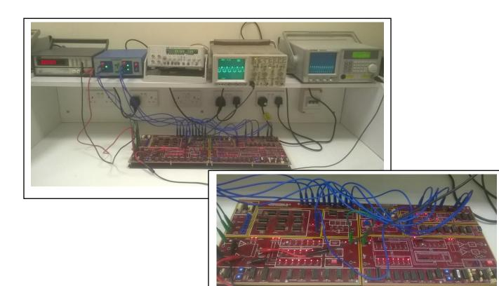
Communications lab provides the students with the fundamental knowledge of communications lab devices and instruments. The construction of different types of transmitters and receivers are explained. Different types of modulation and demodulation is also investigated such as AM, FM, PCM, ASK and FSK.
